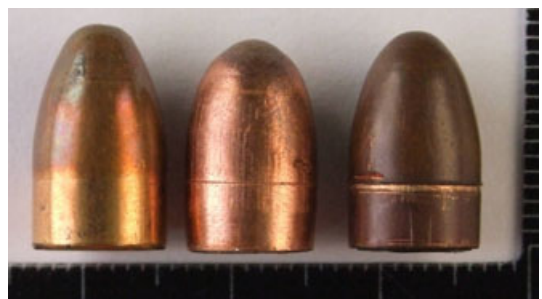
FIG. 3—The appearance of a GW bullet (left), an IW bullet (middle), and an IA bullet (right).
