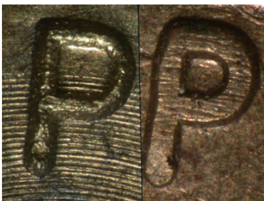
FIG. 8—Head stamp comparison of IA (left) and GA (right) cartridge cases.
