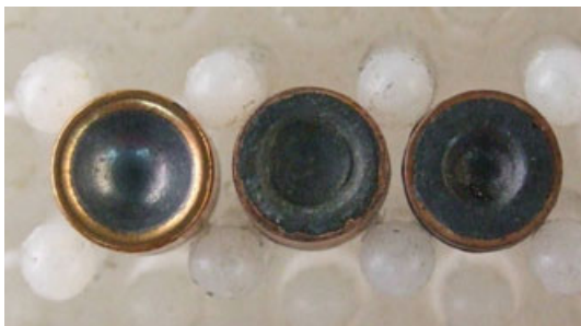
FIG. 4—The bullet base of a GW bullet (left), an IW bullet (middle), and an IA bullet (right).
